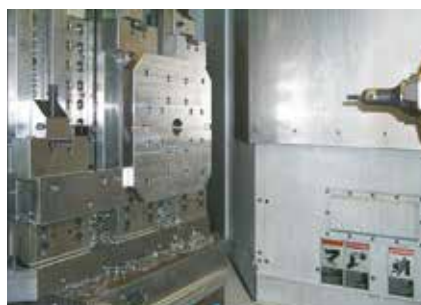
Morse STD montate verticalmente STD vises vertically assembled
