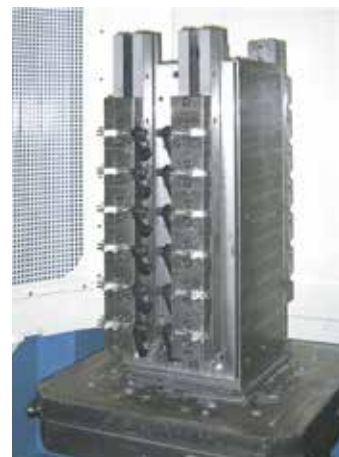
Cubo per piastre riportate con montate piastre e morse MULTIFLEX in verticale Tombstone with modular plates and MULTIFLEX vises vertically assembled
