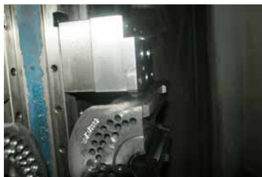
Morse FMS montate verticalmente a triangolo per serrare particolari semitondi/stampi 3pcs. FMS vise vertically mounted in a triangle in order to clamp round workpieces/modules
